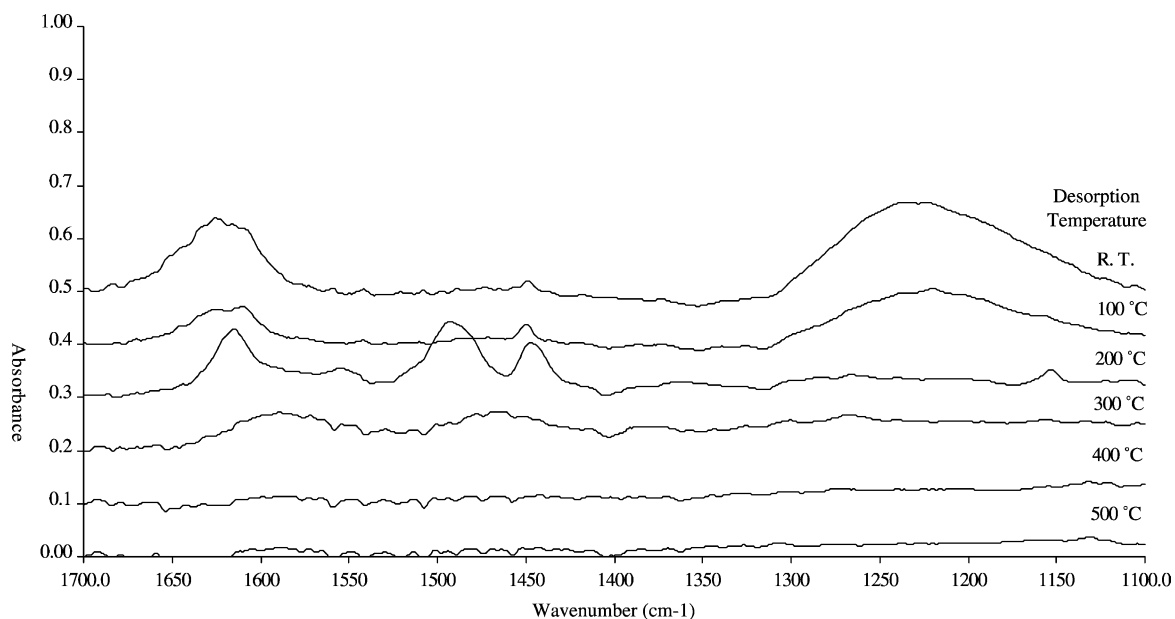
Fig. 5. Spectra of ammonia adsorbed on Cu/alumina calcined at 700 °C, desorbed at various temperatures. Spectra has been offset for clarity (R.T.: room temperature).
